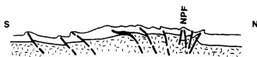
Fig. 1. Section through the Pyrenees (after Choukroune 1974) showing N- and S-directed thrusts rooting steeply into the North Pyrenean Fault (NPF). Hercynian basement is decorated.
